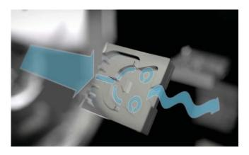
Each channel is designed to create a vortex that oscillates water and sculpts it as it exits into a wave pattern that provides a dense, concentrated spray-to give the feeling of an indulgent shower, without wasting water.
