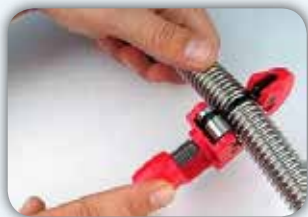
Hose is cut in needed length.
