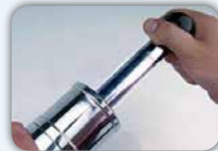
The convolution is flattened by pulling and releasing the equipment as shown in the figure.
