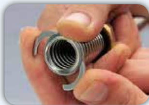
The ring is tightened and fixed behind the flattened convolution.
